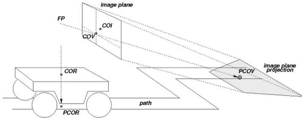
Figure 2. Projection of image plane on the ground plane and location of salient points for performance evaluation
