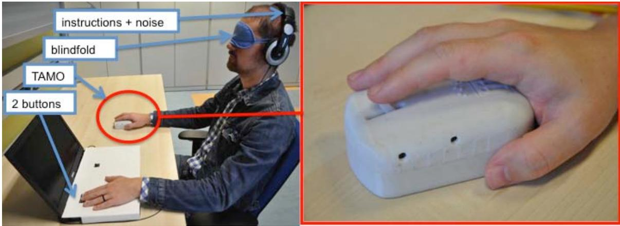
Figure 2: Experimental setup: subject interacting with the single taxel of the TAMO device
