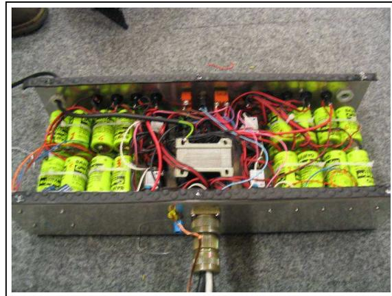
Fig. 11: Inside of the power supply box: from the 8 groups of 4 batteries the power supply passes through the red and violet cables, placed on purpose in those positions. The transformer, which provides power supply for the digital part (in acquisition state) and recharges the batteries (in recharging state), appears in the center of the box.
